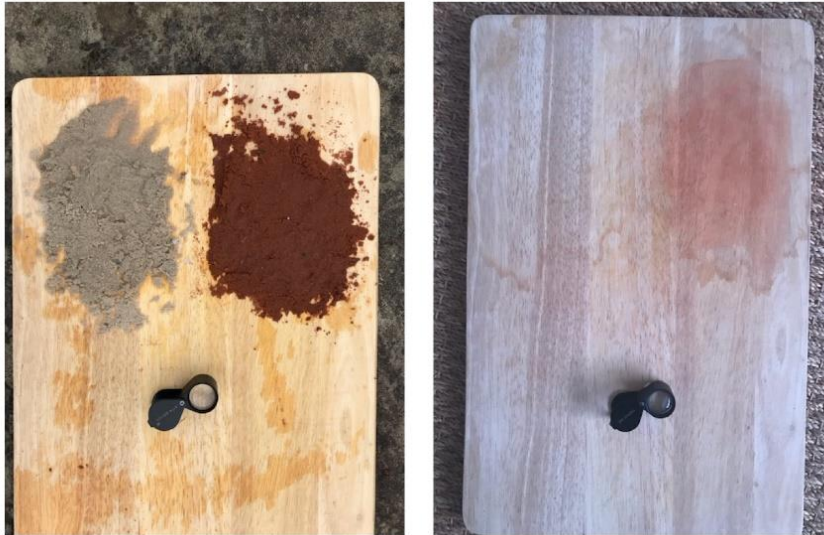
Picture 10. Left board, damp white and red sand. Right board, after 24 hours, red stain left after removing sand
